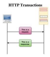
The above figure shows the HTTP transaction between client and server. The client initiates a transaction by sending a request message to the server. The server replies to the request message by sending a response message.
