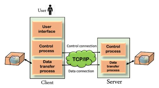
The above figure shows the basic model of the FTP. The FTP client has three components: the user interface, control process, and data transfer process. The server has two components: the server control process and the server data transfer process.
