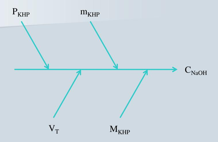
Simple cause and effect diagram for standardization of a NaOH solution with KHP
